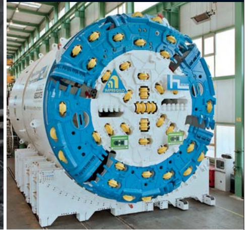
BELOW: VTC's state-of-the-art 23.5ft (7.2m) diameter Herrenknecht Mixshield, designed with a maximum closed-mode operating pressure of 17 bar
