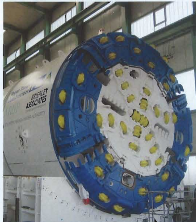
» Vegas Tunnel Constructors is digging a 600-foot shaft and will use a specialized Herrenknecht tunnel-boring machine designed to operate in high water pressure to drive the three-mile tunnel. The intake structure will be constructed on a barge at the shoreline and then lowered into a hole created by the use of explosives.
